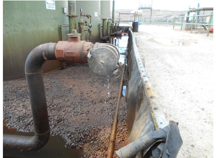
Leak at offload connection
