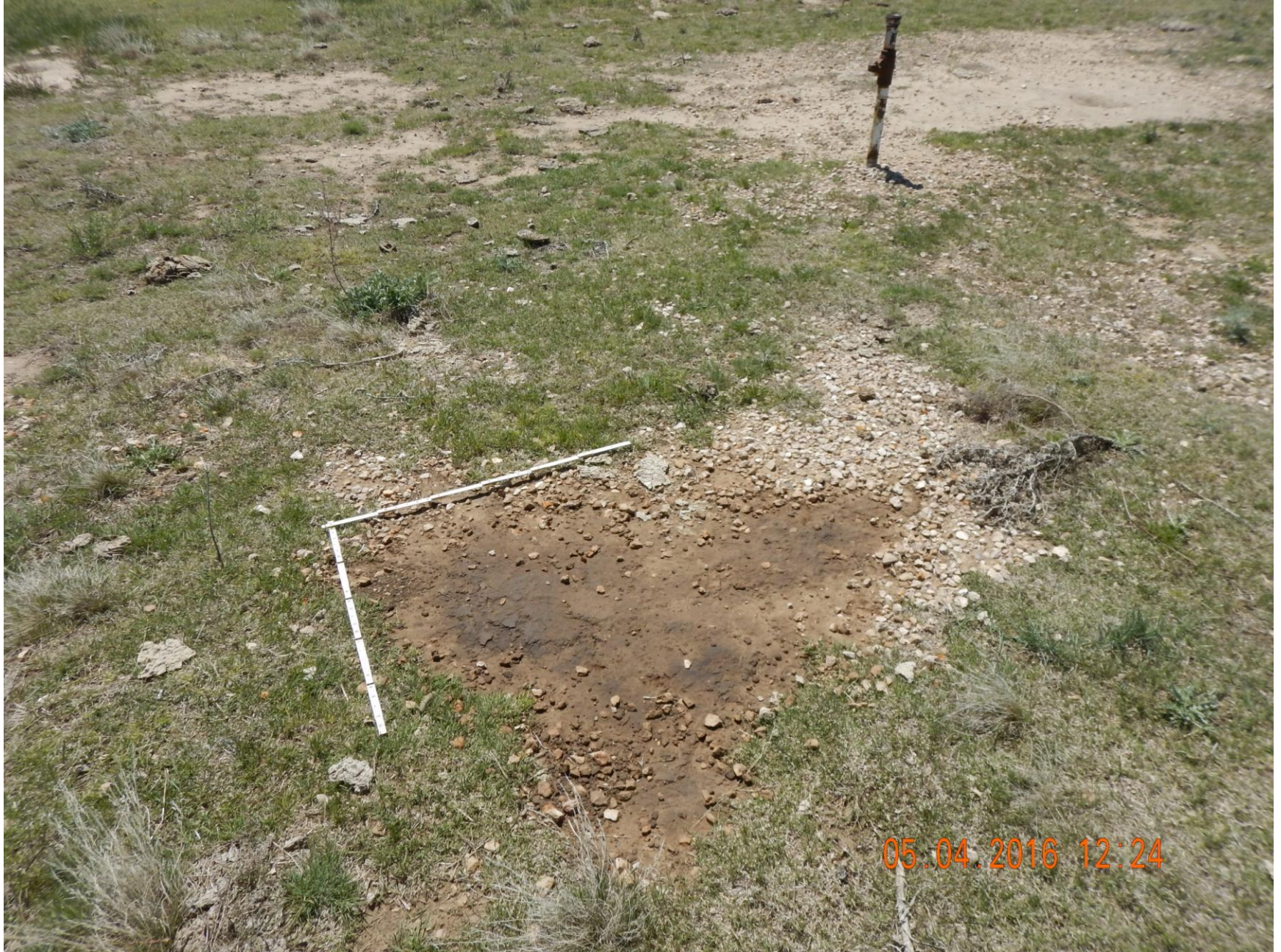
Figure 3: Photo taken from the north end of the location. Photo shows impacted soils and riser. 3'x2' measuring stick for reference.
