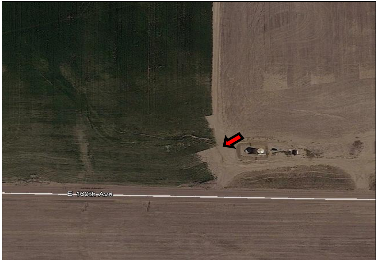
Photo 1: Aerial imagery illustrating erosion initiates on the tank battery location, traveling west onto cropland.
