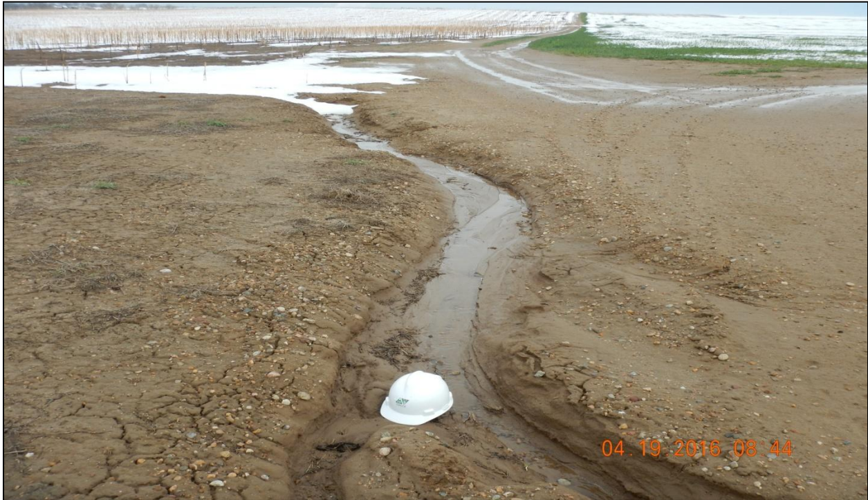
Photo 6: Photo taken 4/19/16 west of tank battery location, facing North. Erosion continues north approximately 50 feet, then heads west onto cropland (see next photo).
