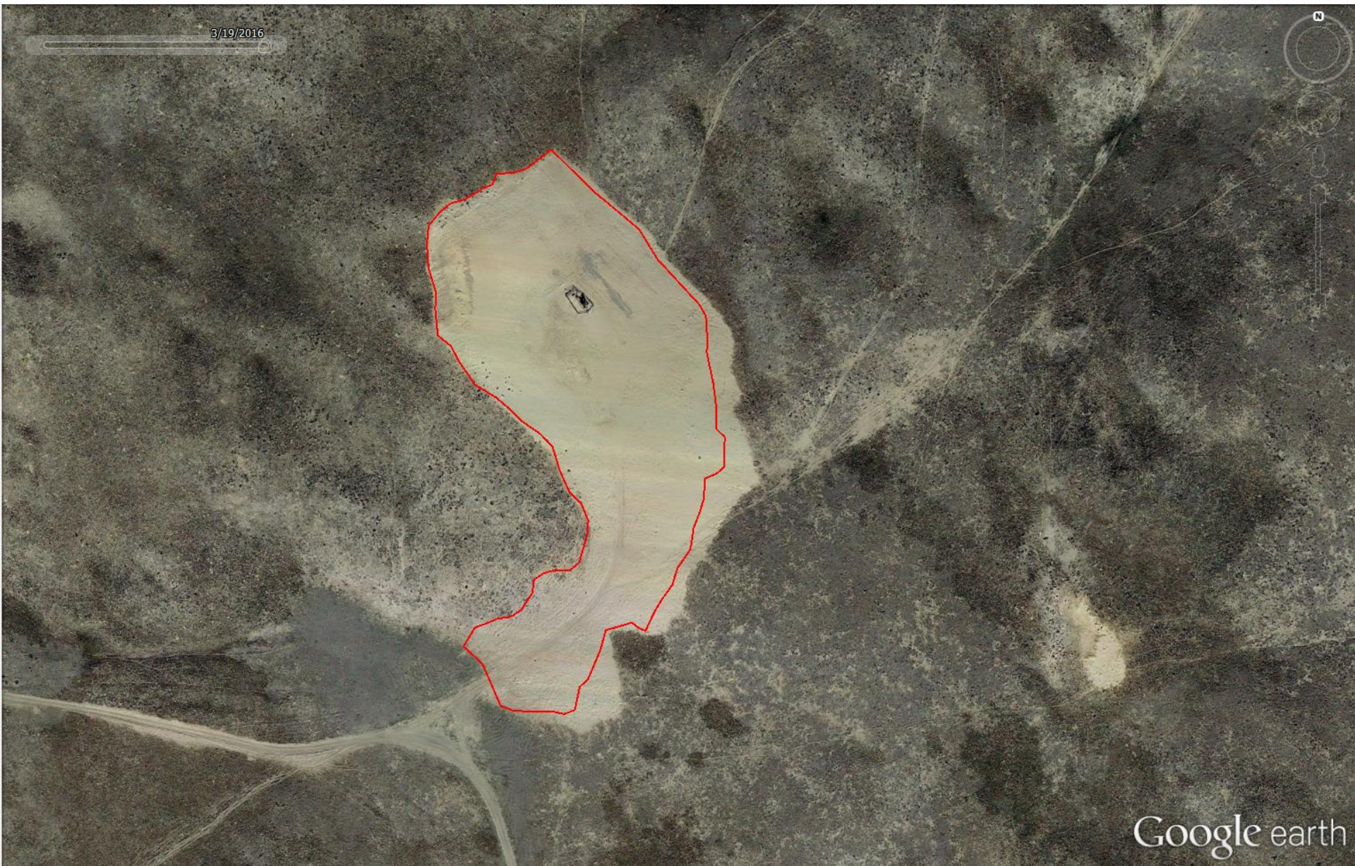
Figure 12: 2016 Aerial imagery. Image shows locations current size of disturbance compared to 2015 (red line). Note locations current area of disturbance has not been reduced in size as required by interim reclamation rules, but rather, has increased in size.
