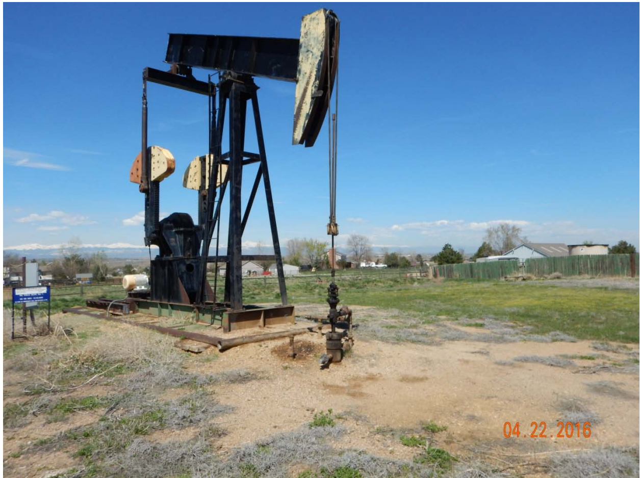
Figure 3 - Oil-stained soil at wellhead.
