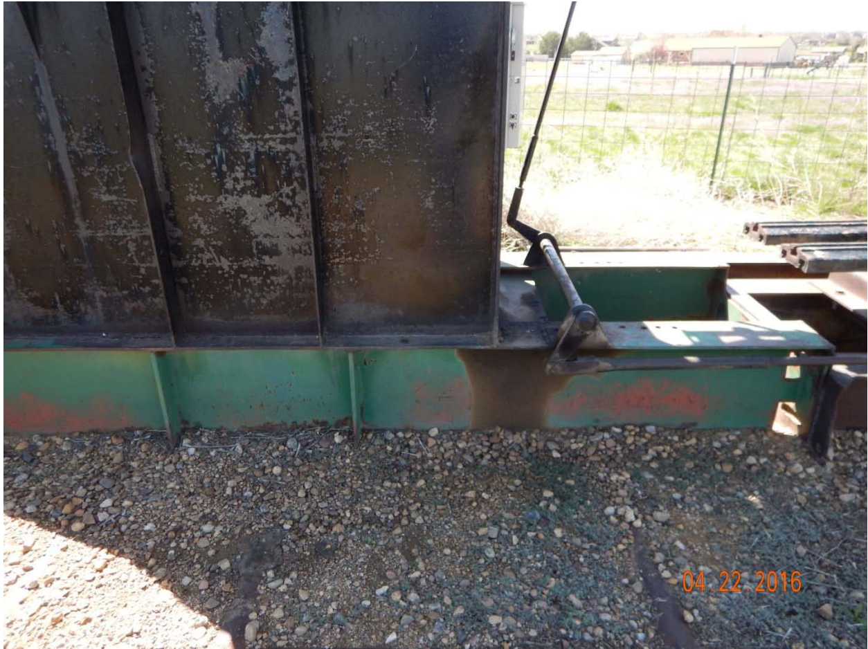
Figure 4 - Grease stain on base of pump jack.
