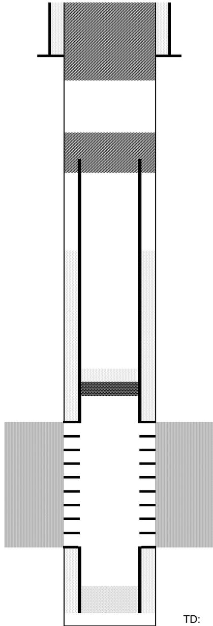
Cut surface casing off 6'-8' below surface.
