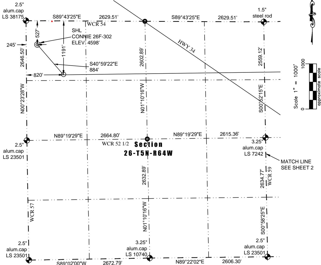
In accordance with a request from Barney Hammond of PDC Energy, Inc., Washburn Land Surveying, LLC has determined the location of the **CONNIE 26F-302** well site to be SHL: 527' FNL and 245' FWL, (BHL: 1160' FNL and 500' FEL), as measured at ninety (90) degrees from the section lines of Sections 26 and 25, Township 5 North, Range 64 West of the 6th Principal Meridian, Weld County Colorado.
