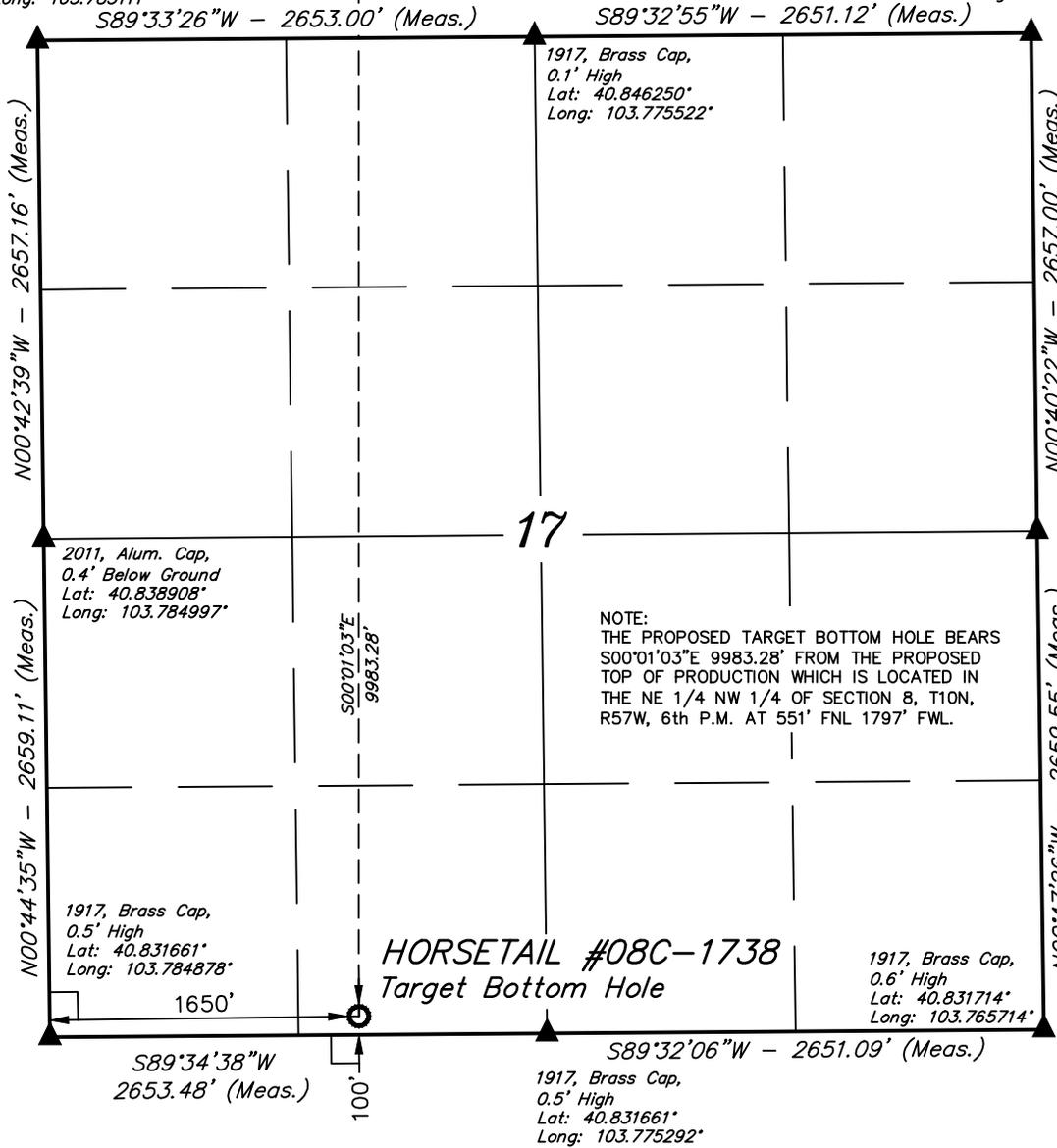
Well location, HORSETAIL #08C-1738 (TARGET BOTTOM HOLE), located as shown in the SE 1/4 SW 1/4 of Section 17, T10N, R57W, 6th P.M., Weld County, Colorado.
