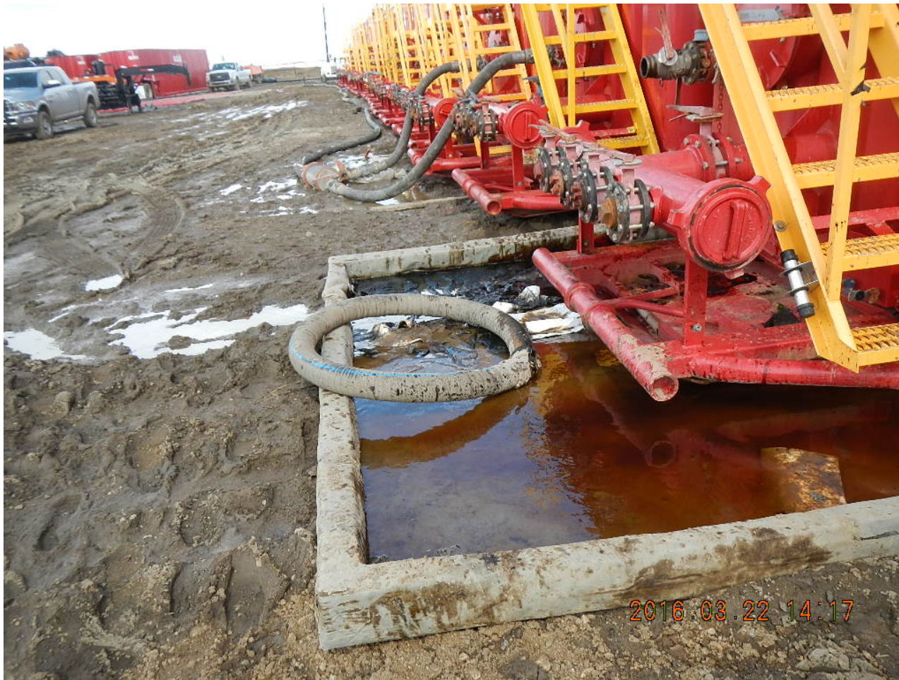
Secondary containment, has some residual water from cleaning the secondary containment.
