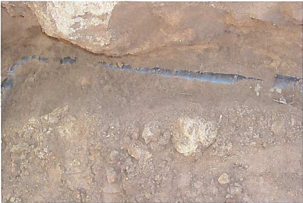
Photo 3 – Looking into test pit 1 at intact DEFS line. No staining or odors were noted.
