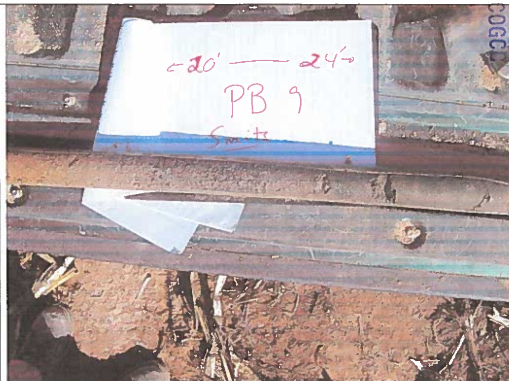
PB9 core 20-24', with visible staining at 22.5-24 ft. Sample moist/wet below 22.5'
