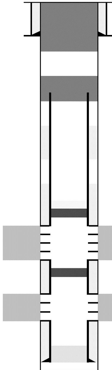
Cut surface casing off 6'-8' below surface.
