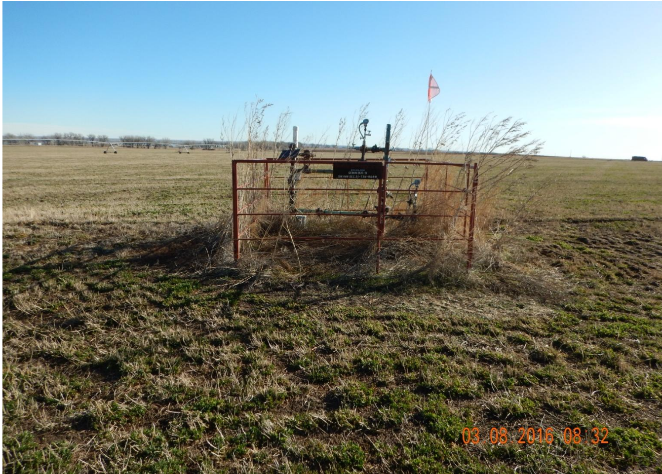
Photo 2. Photo taken from west of location, facing East. Remove weeds around wellhead. Weeds within 25 feet of operating oil and gas equipment are a potential safety or fire concern.
