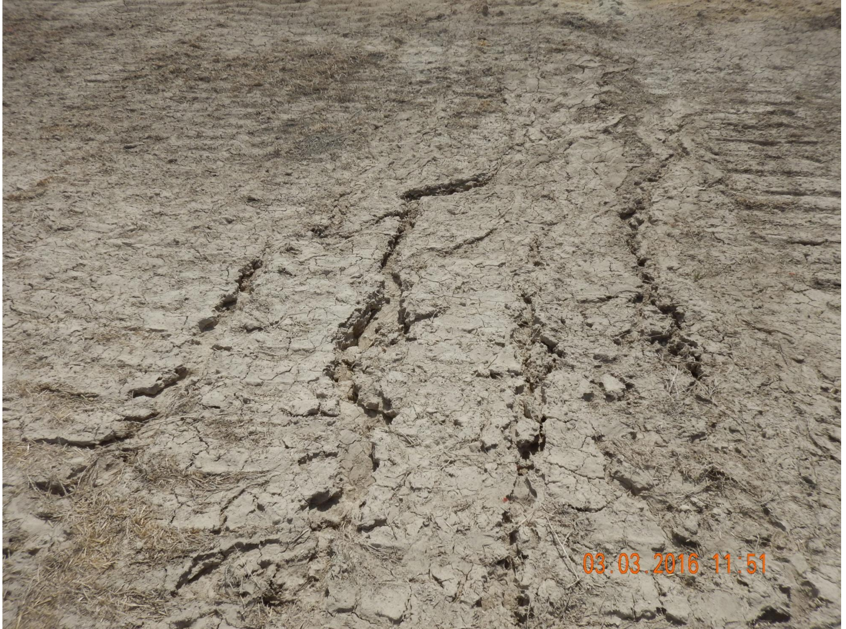
Figure 13: Photo taken from the north end of the location. Photo show rill erosion on slope.
