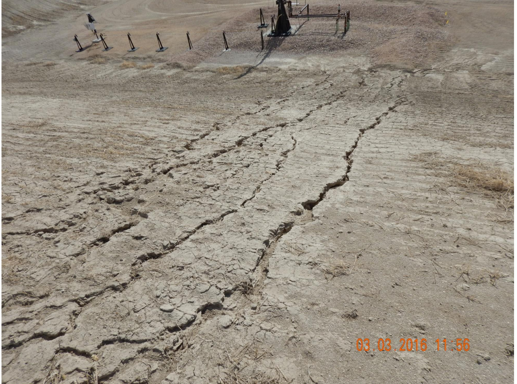
Figure 21: Photo taken from the north end of the location, facing south. Photo of rill erosion on slope, and sediment deposition on location.
