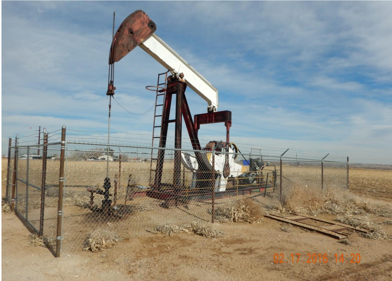
Photo 3. Photo taken from southern location, facing Northeast. Need to remove weeds around all operating oil and gas equipment on location.
