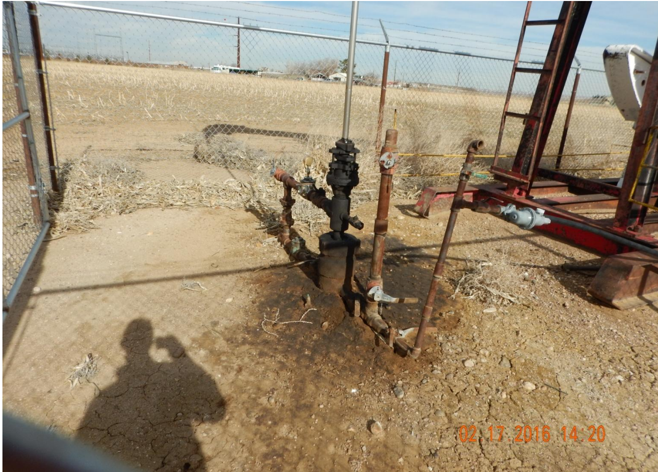
Photo 4. Photo taken from pump jack, looking at the wellhead. Remove or remediate stained soil (<1 bbl) around wellhead.
