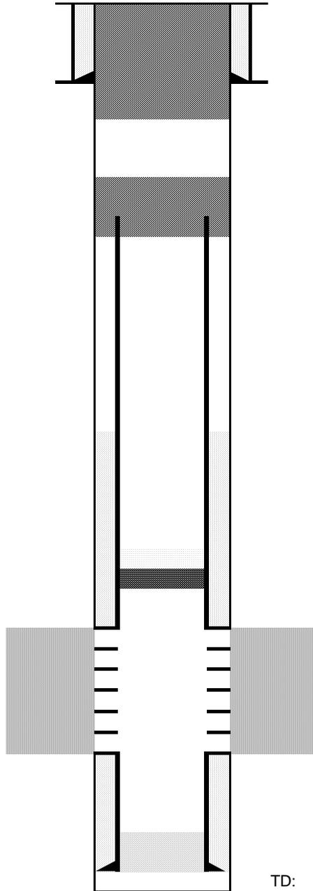
Cut surface casing off 6'-8' below surface.
