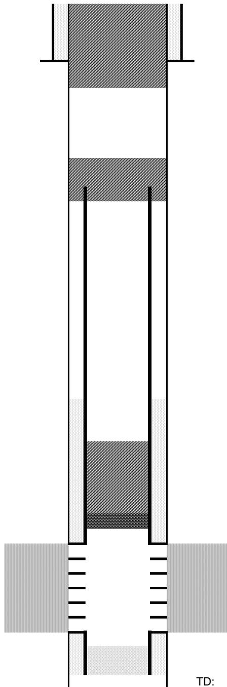
Cut surface casing off 6'-8' below surface.
