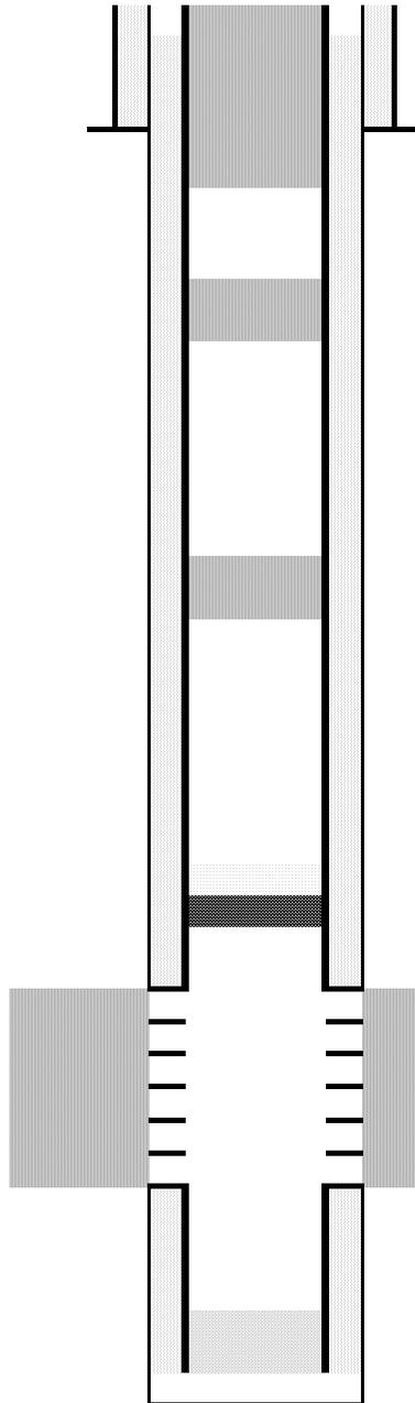
Cut surface casing off 6'-8' below surface.
