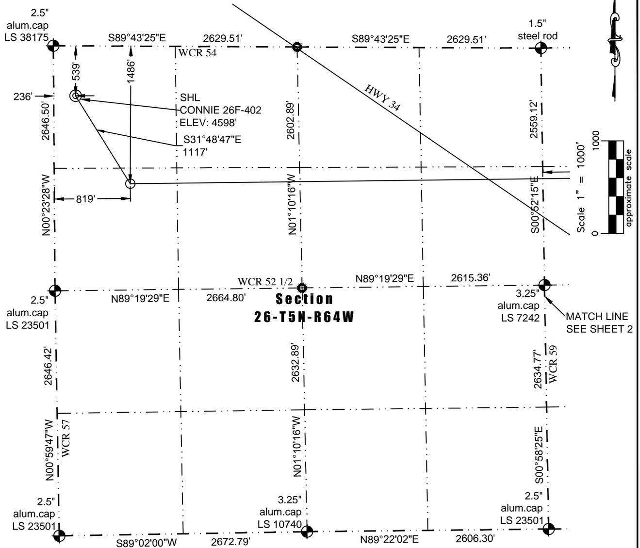
In accordance with a request from Barney Hammond of PDC Energy, Inc., Washburn Land Surveying, LLC has determined the location of the **CONNIE 26F-402** well site to be SHL: 539' FNL and 236' FWL, (BHL: 1433' FNL and 2140' FWL), as measured at ninety (90) degrees from the section lines of Sections 26 and 25, Township 5 North, Range 64 West of the 6th Principal Meridian, Weld County Colorado.
