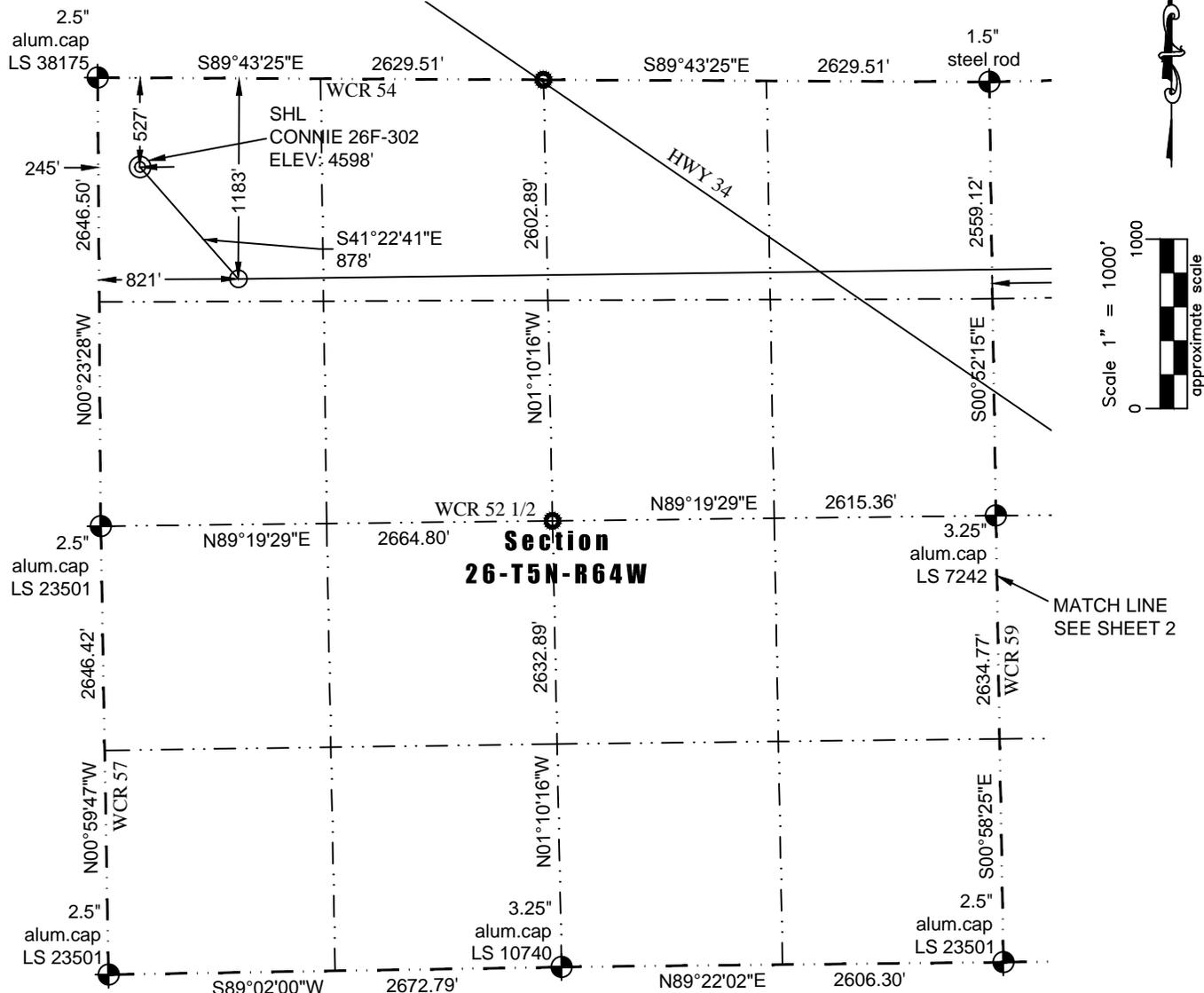
In accordance with a request from Barney Hammond of PDC Energy, Inc., Washburn Land Surveying, LLC has determined the location of the **CONNIE 26F-302** well site to be SHL: 527' FNL and 245' FWL, (BHL: 1130' FNL and 2140' FWL), as measured at ninety (90) degrees from the section lines of Sections 26 and 25, Township 5 North, Range 64 West of the 6th Principal Meridian, Weld County Colorado.
