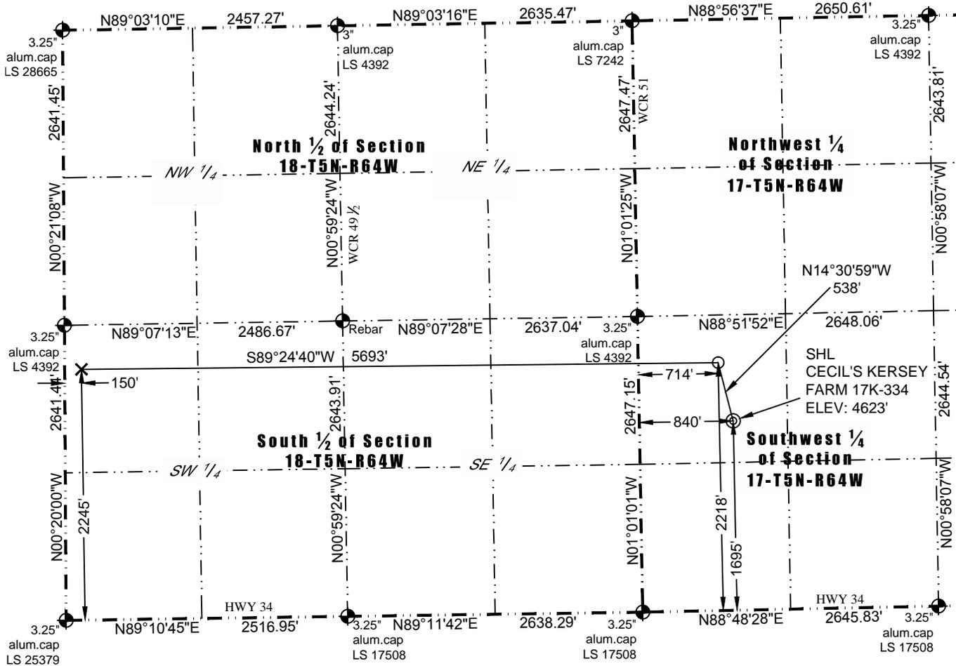
In accordance with a request from Barney Hammond of PDC Energy, Inc., Washburn Land Surveying, LLC has determined the location of the **CECIL'S KERSEY FARM 17K-334** well site to be SHL: 1695' FSL and 840' FWL, (BHL: 2245' FSL and 150' FWL), as measured at ninety (90) degrees from the section lines of Sections 17 and 18, Township 5 North, Range 64 West of the 6th Principal Meridian, Weld County Colorado.
