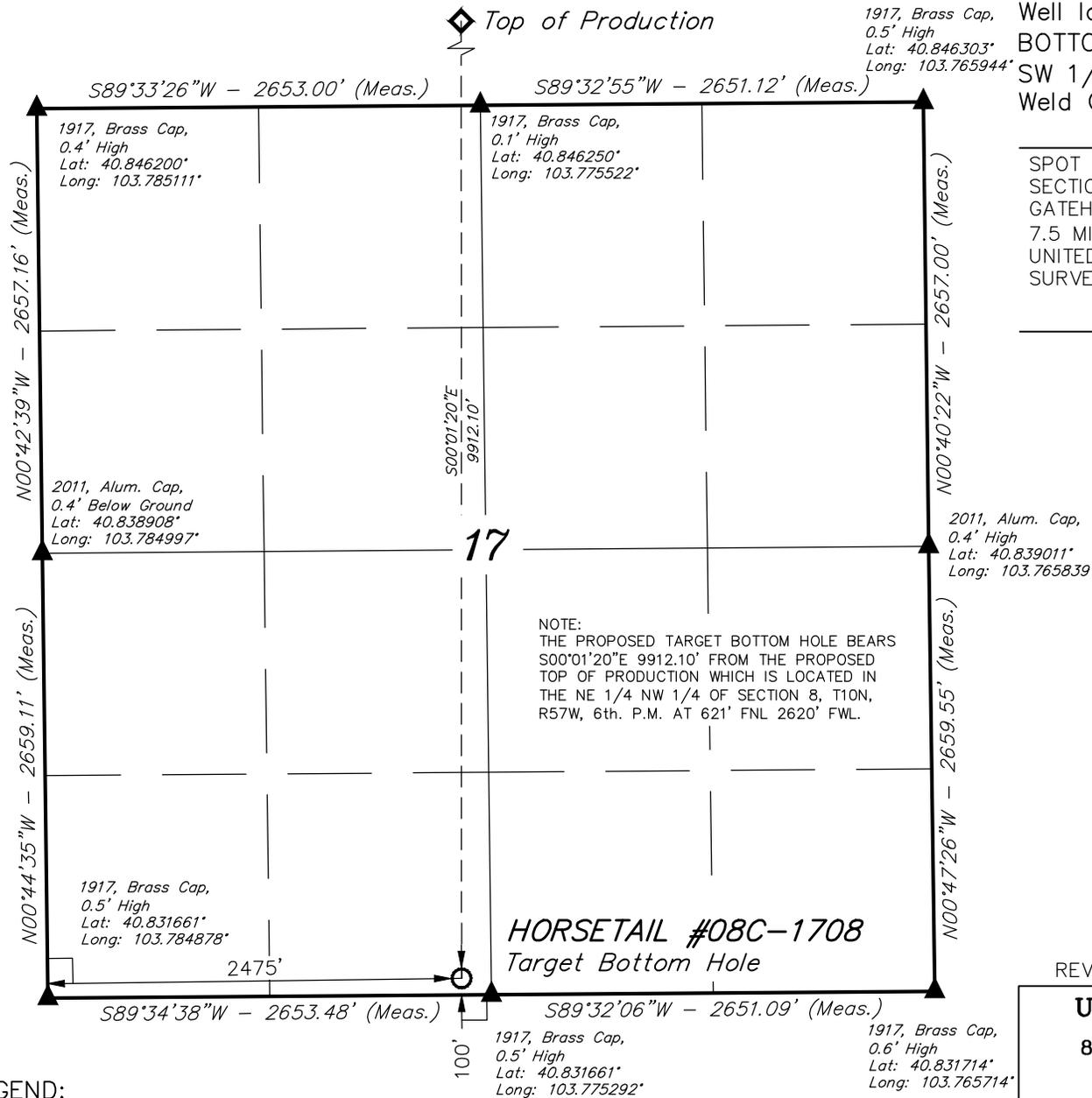
Well location, HORSETAIL #08C-1708 (TARGET BOTTOM HOLE), located as shown in the SE 1/4 SW 1/4 of Section 17, T10N, R57W, 6th. P.M., Weld County, Colorado.
