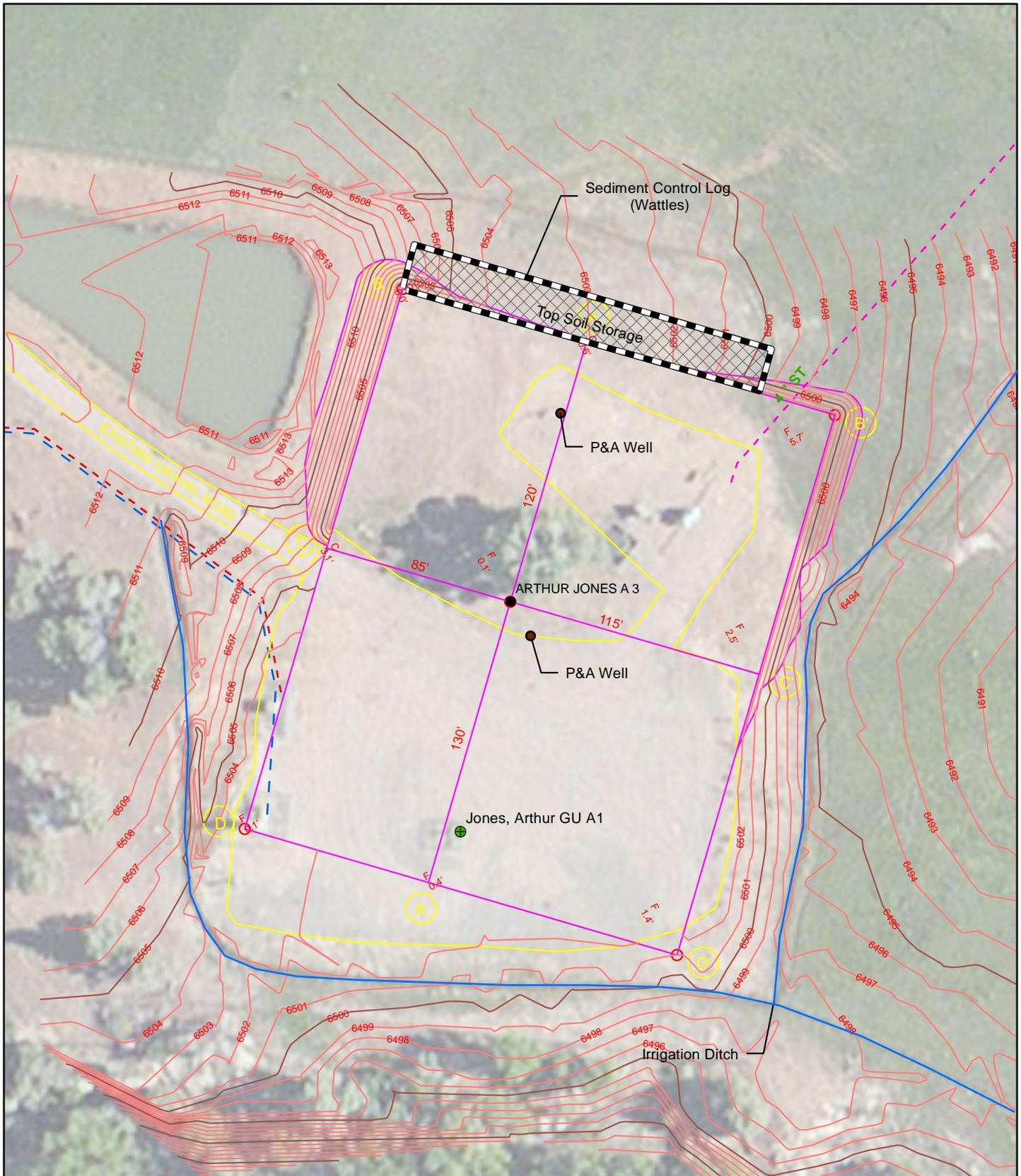
**Note: Location will be bermed during construction/drilling**
