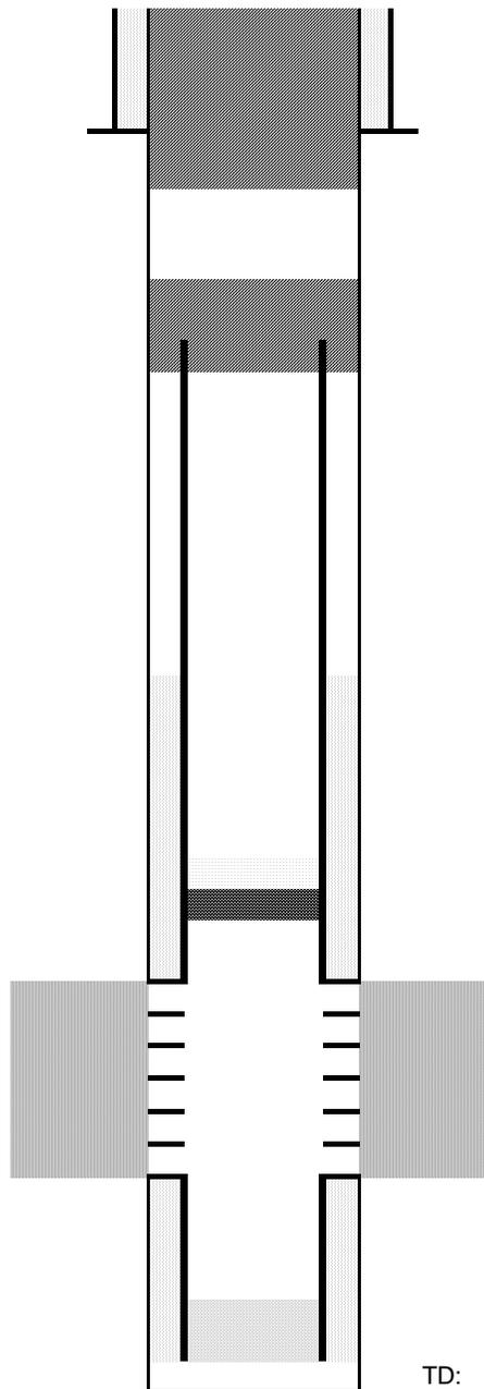
Cut surface casing off 6'-8' below surface.
