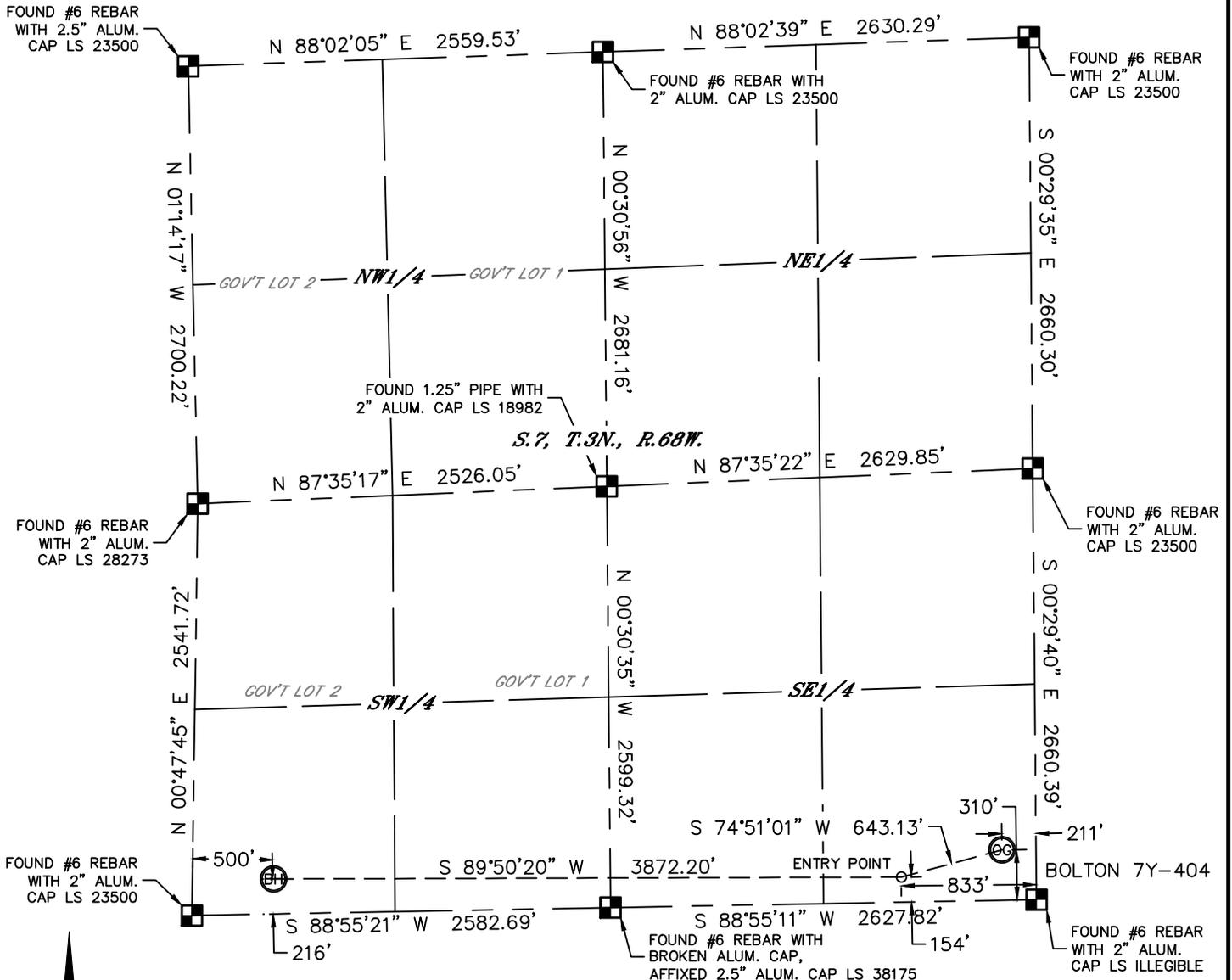
In accordance with a request from Jake Bragg with PDC ENERGY, INC. Lat40°, Inc. has determined the surface location of the BOLTON 7Y-404 to be 310' from the SOUTH line and 211' from the EAST line and the bottom hole to be 216' from the SOUTH line and 500' from the WEST line as measured at right angles from the section lines of Section 7, Township 3 North, Range 68 West of the Sixth Principal Meridian, County of Weld, State of Colorado.
