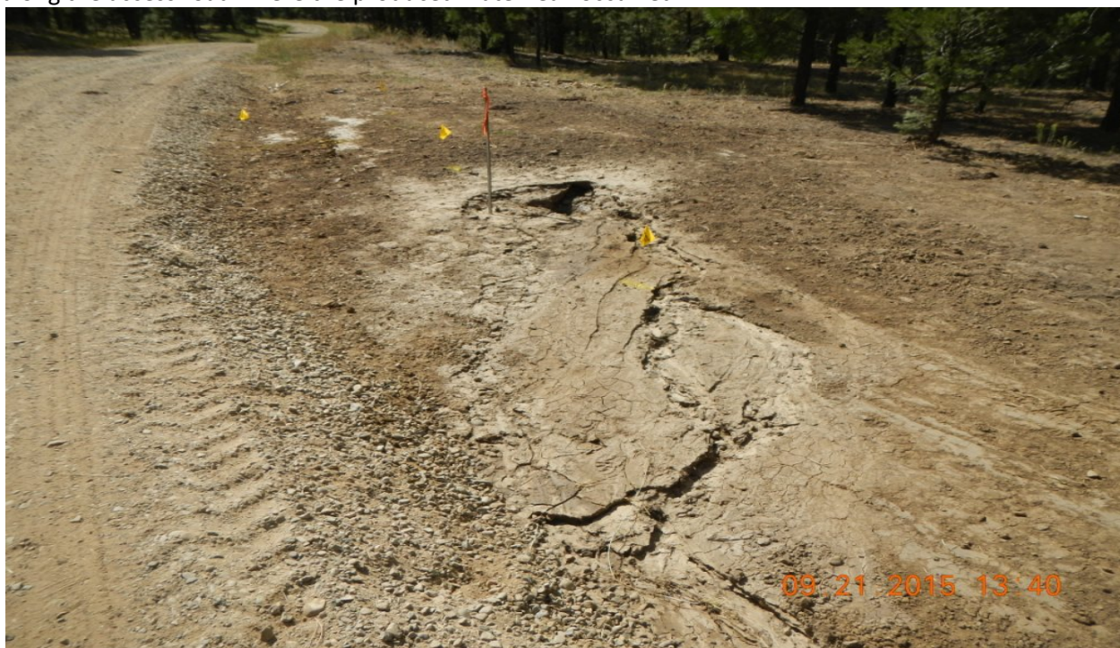
photo 2: North side of the access road where produced water leak occurred.
