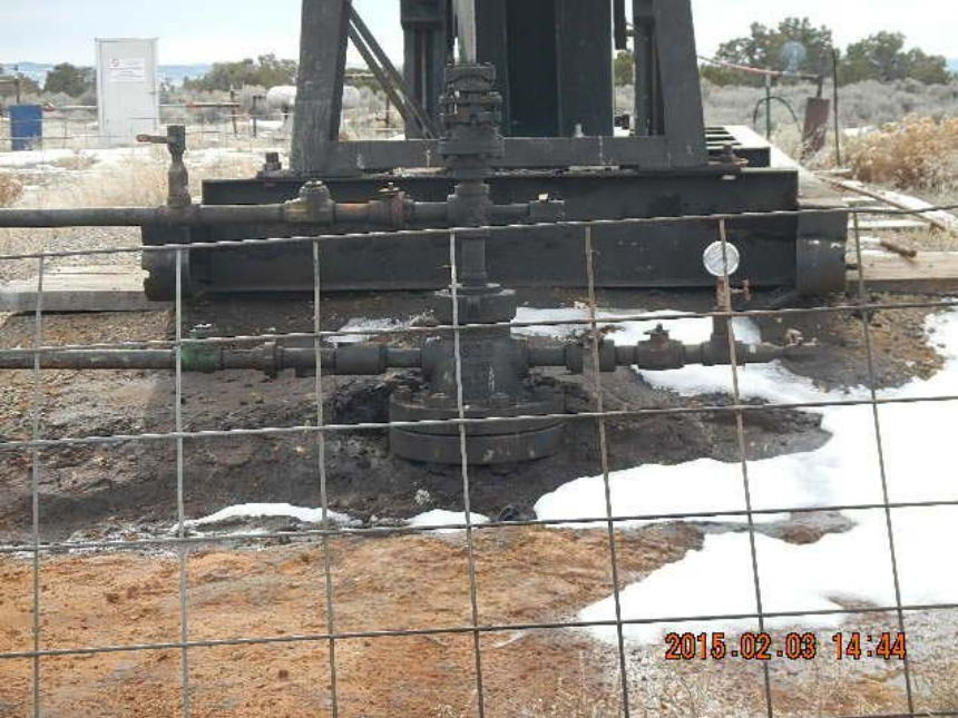
Stained soil at wellhead – initial inspection
