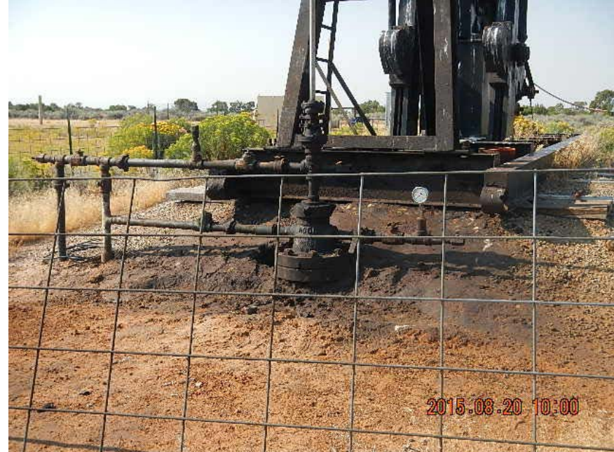
Stained soil at wellhead – follow up inspection
