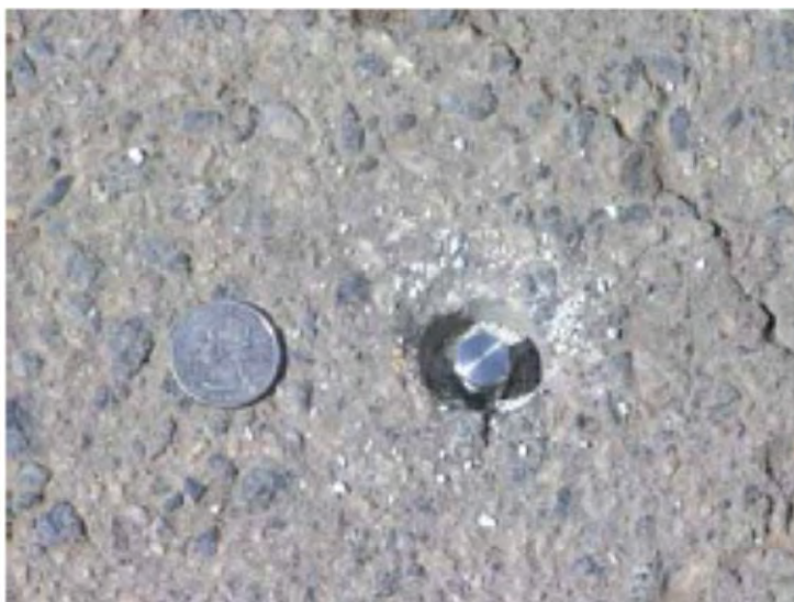
Example of flush mounted vapor sampling point
