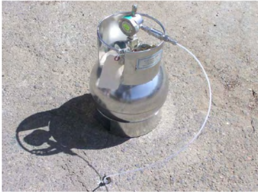
Example of the flush mounted vapor sampling point
