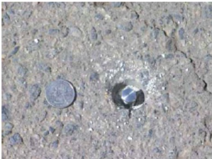
Example of flush mounted vapor sampling point
