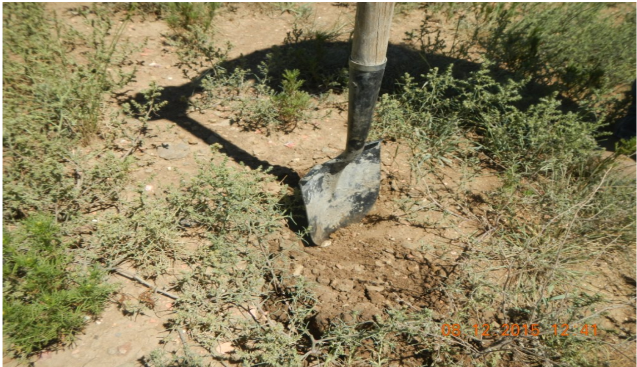
photo 3: : Areas of the initial 200' of access road seem to have compacted soils.
