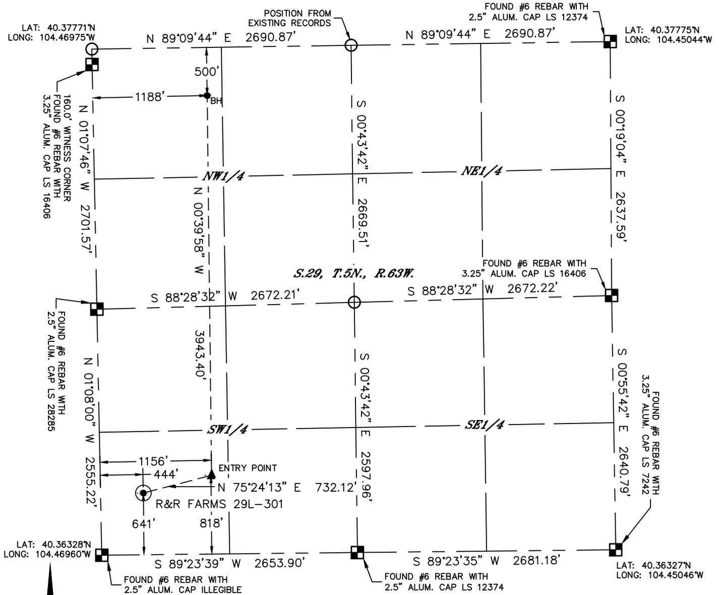
In accordance with a request from Jeff Dillingham with PDC ENERGY, INC. Lat40°, Inc. has determined the surface location of the R&R FARMS 29L-301 to be 641' from the SOUTH line and 444' from the WEST line and the bottom hole to be 500' from the NORTH line and 1188' from the WEST line as measured at right angles from the section lines of Section 29, Township 5 North, Range 63 West of the Sixth Principal Meridian, County of Weld, State of Colorado.
