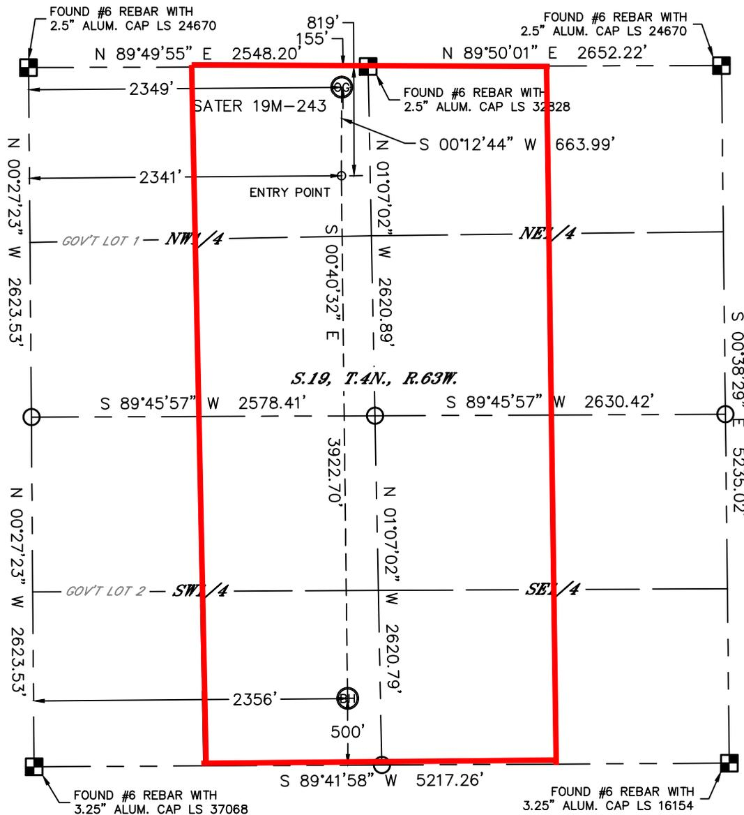
In accordance with a request from Mac Neumann with PDC ENERGY Lat40°, Inc. has determined the surface location of the SATER 19M-243 to be 155' from the NORTH line and 2349' from the WEST line and the bottom hole to be 500' from the SOUTH line and 2356' from the WEST line as measured at right angles from the section lines of Section 19, Township 4 North, Range 63 West of the Sixth Principal Meridian, County of Weld, State of Colorado.
