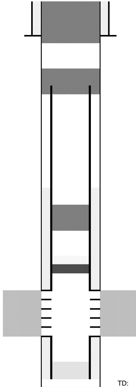
Cut surface casing off 6'-8' below surface.
