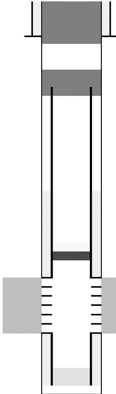
Cut surface casing off 6'-8' below surface.
