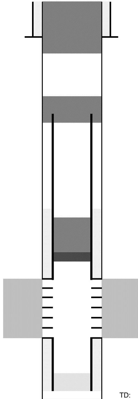
Cut surface casing off 6'-8' below surface.
