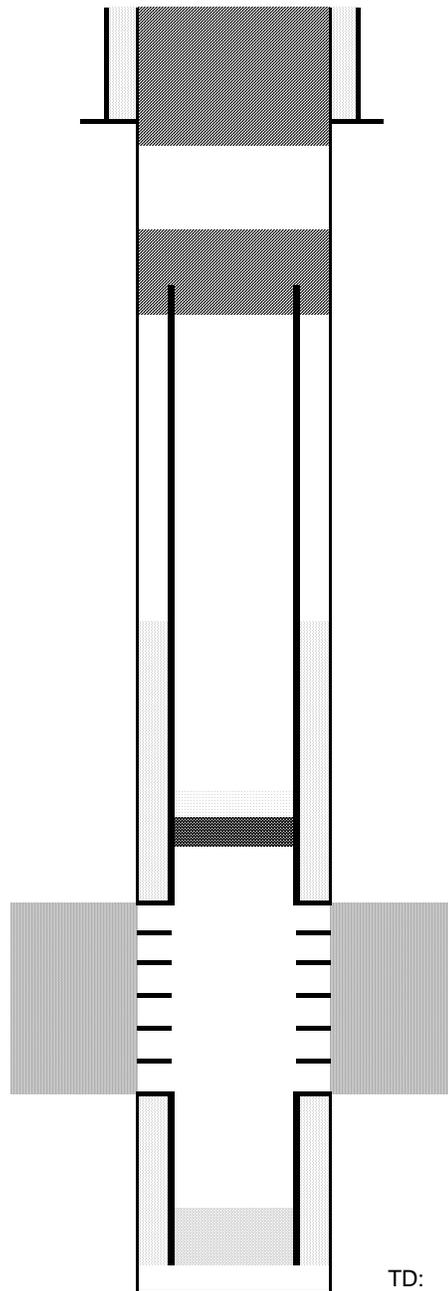
Cut surface casing off 6'-8' below surface.
