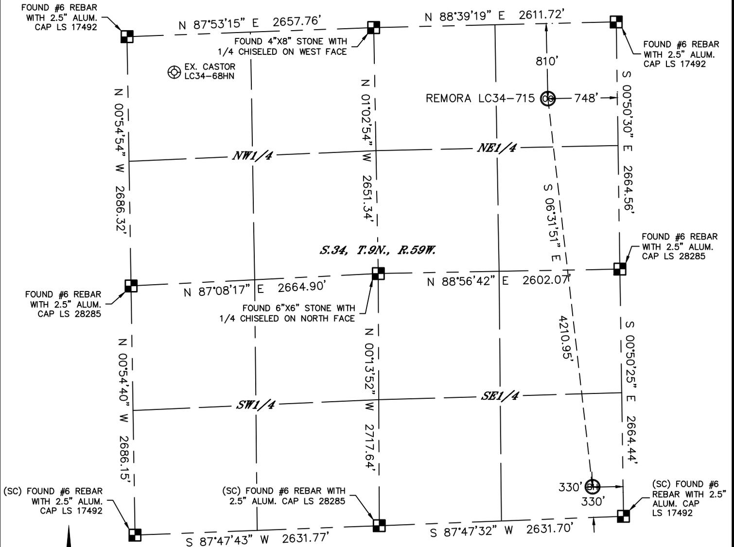
In accordance with a request from Brian James with Noble Energy Inc. Lat40°, Inc. has determined the surface location of the REMORA LC34-715 to be 810' from the NORTH line and 748' from the EAST line and the bottom hole to be 330' from the SOUTH line and 330' from the EAST line as measured at right angles from the section lines of Section 34, Township 9 North, Range 59 West of the Sixth Principal Meridian, County of Weld, State of Colorado.
