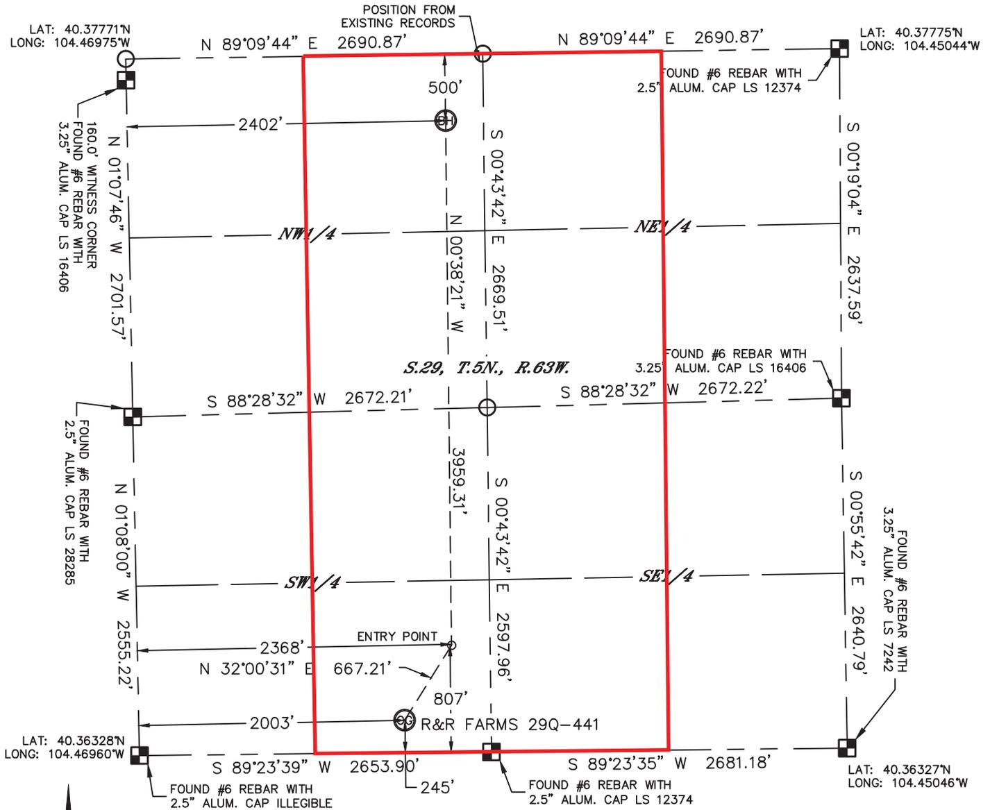
In accordance with a request from Thomas Bragg with PDC ENERGY, INC. Lat40°, Inc. has determined the surface location of the R&R FARMS 29Q-441 to be 245' from the SOUTH line and 2003' from the WEST line and the bottom hole to be 500' from the NORTH line and 2402' from the WEST line as measured at right angles from the section lines of Section 29, Township 5 North, Range 63 West of the Sixth Principal Meridian, County of Weld, State of Colorado.
