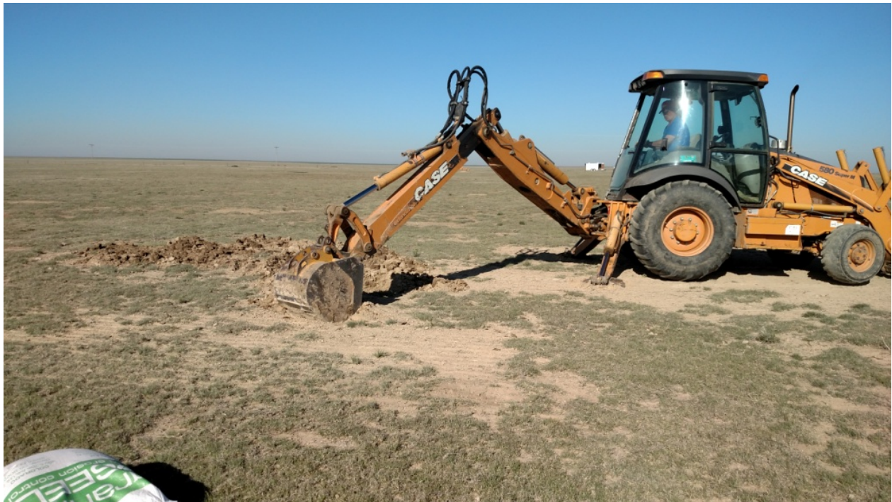
photo 5: Soil de-compaction in areas where vegetation will not grow.
