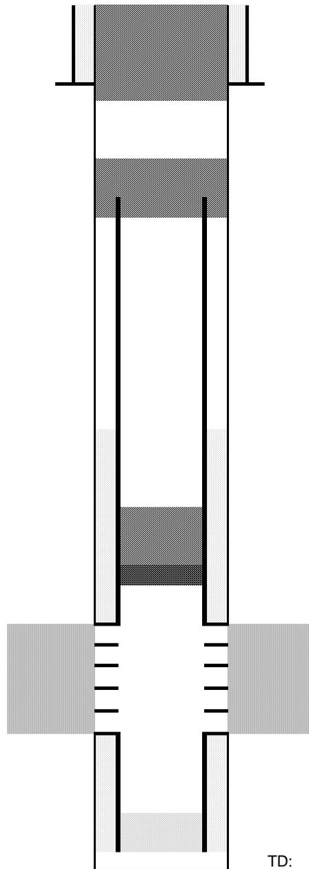
Cut surface casing off 6'-8' below surface.
