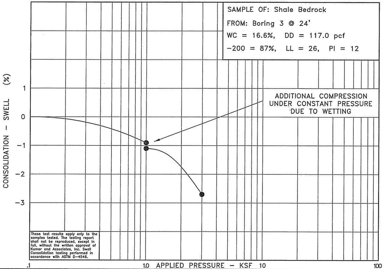
These test results apply only to the samples tested. The testing report shall not be reproduced, except in full, without the written approval of Kumar and Associates, Inc. Swell Consolidation testing performed in accordance with ASTM D-4546.
