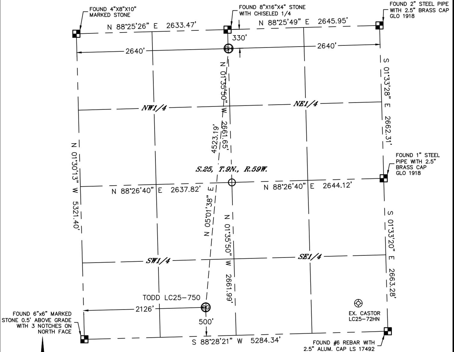
In accordance with a request from Cody Ball with Noble Energy Inc. Lat40°, Inc. has determined the surface location of the TODD LC25-750 to be 500' from the SOUTH line and 2126' from the WEST line and the bottom hole to be 330' from the NORTH line and 2640' from the EAST line as measured at right angles from the section lines of Section 25, Township 9 North, Range 59 West of the Sixth Principal Meridian, County of Weld, State of Colorado.
