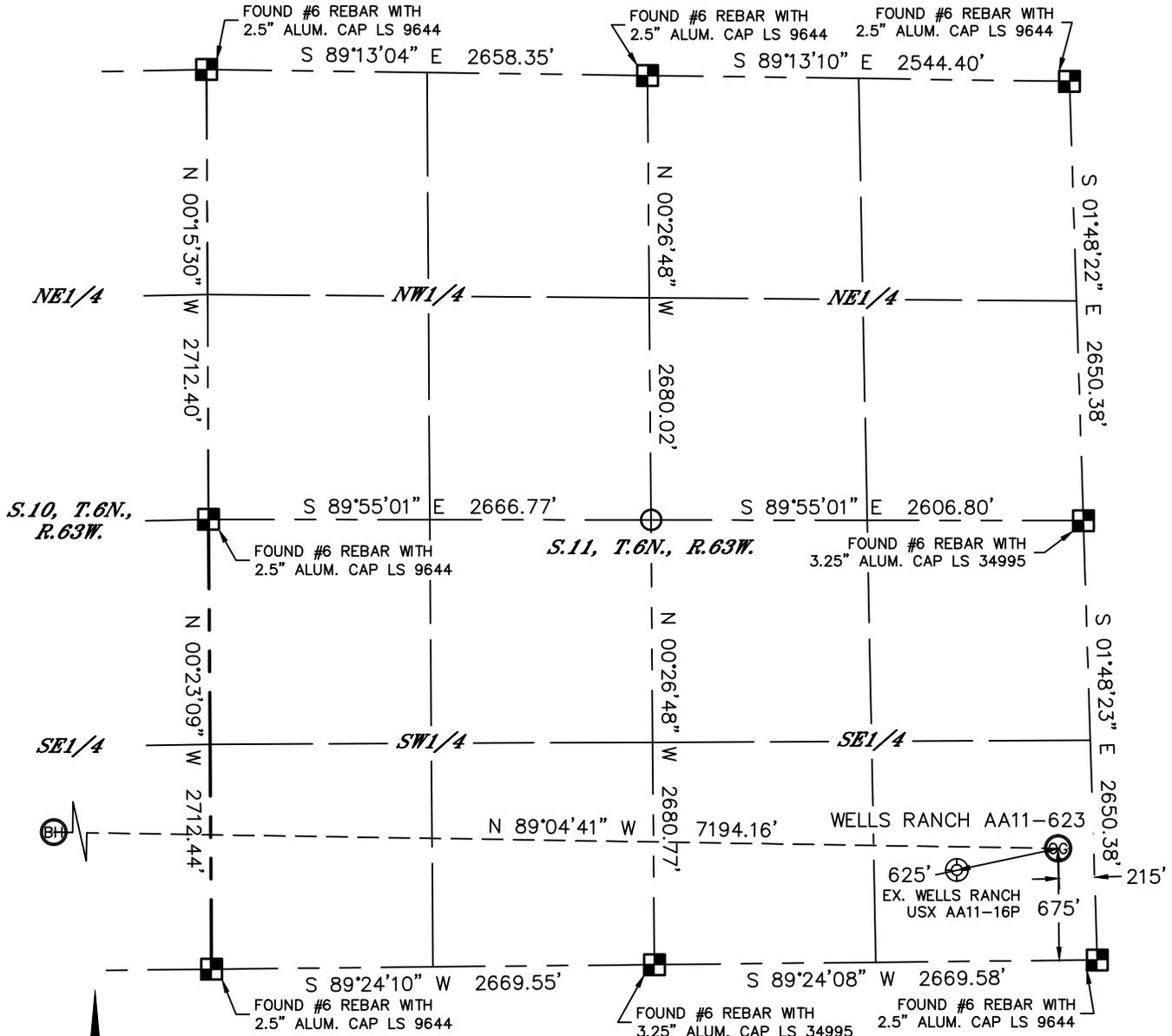
In accordance with a request from Greg Wilson with Noble Energy Inc. Lat40°, Inc. has determined the surface location of the WELLS RANCH AA11-623 to be 675' from the SOUTH line and 215' from the EAST line of Section 11, Township 6 North, Range 63 West and the bottom hole to be 867' from the SOUTH line and 2085' from the EAST line as measured at right angles from the section lines of Section 10, Township 6 North, Range 63 West of the Sixth Principal Meridian, County of Weld, State of Colorado.
