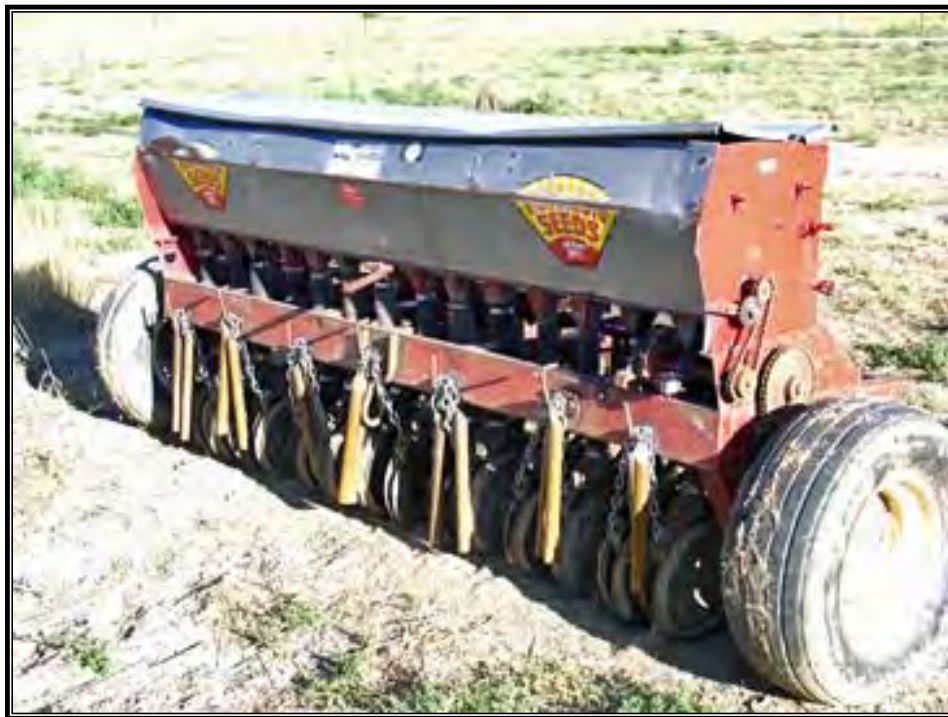
Photo 16: Drag Chains in Transport Position
