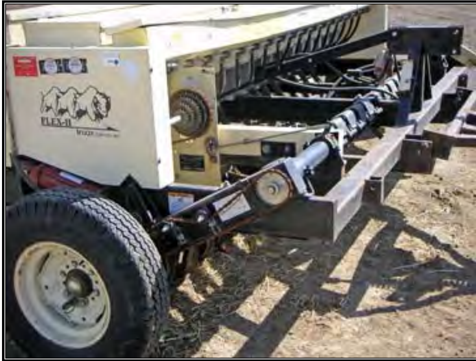
Photo 19: Seed Drill Gear Assembly
