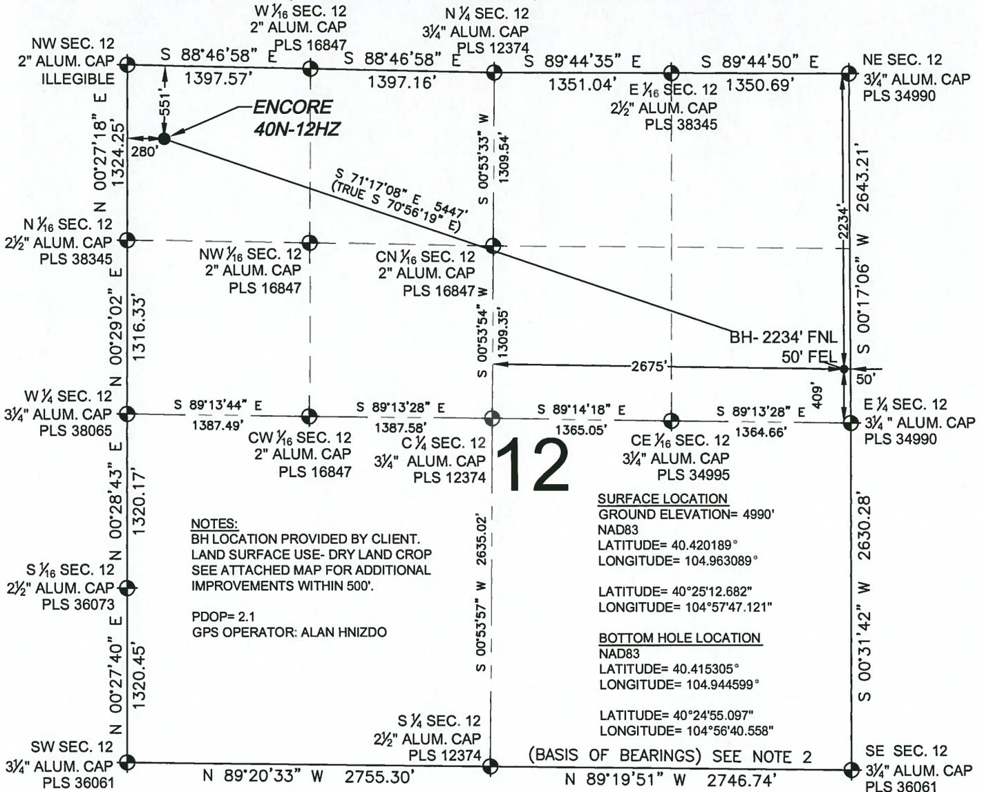
WELL ENCORE 40N-12HZ TO BE LOCATED 551' FNL AND 280' FWL
