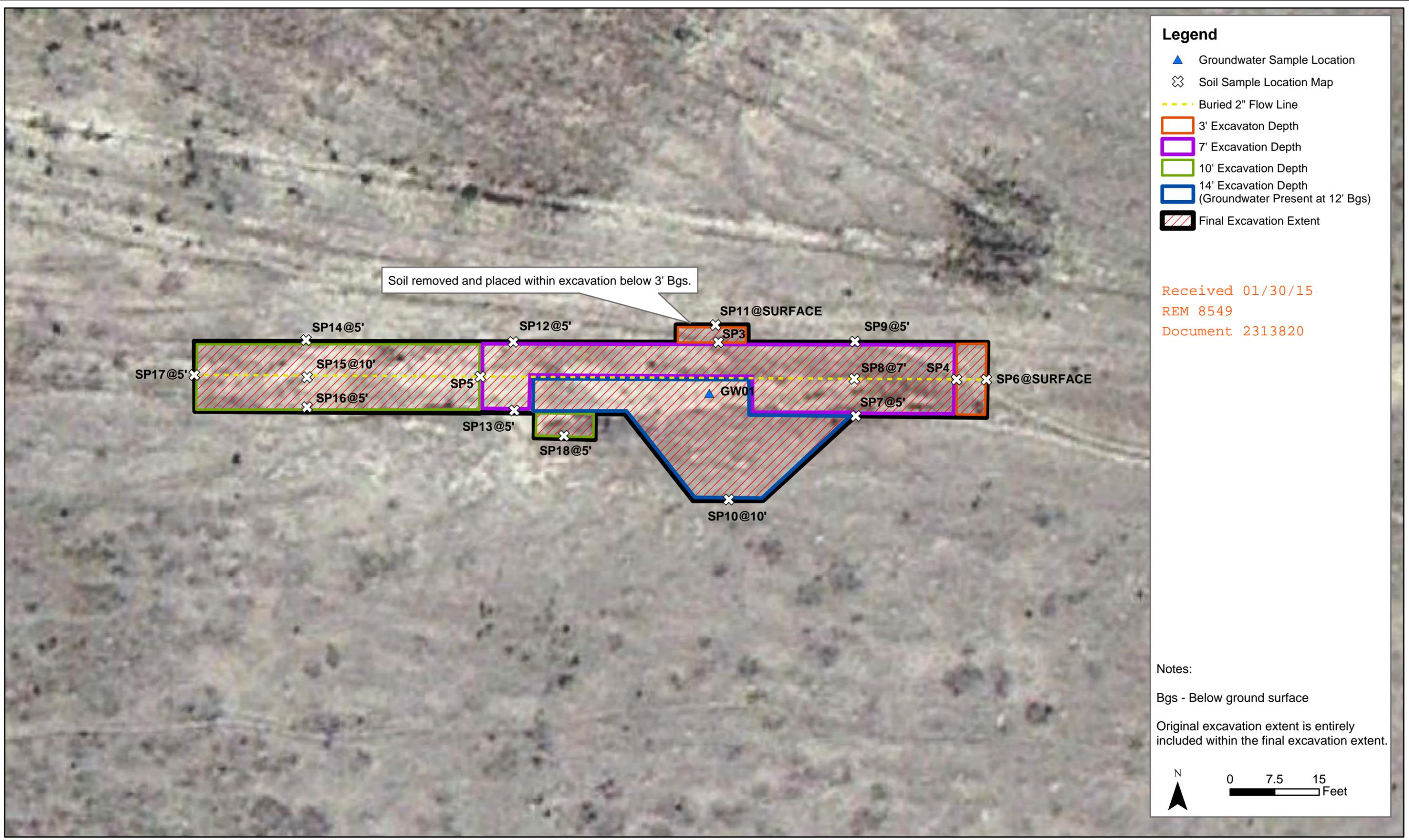
Soil removed and placed within excavation below 3' Bgs.
