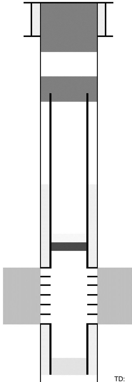
Cut surface casing off 6'-8' below surface.
