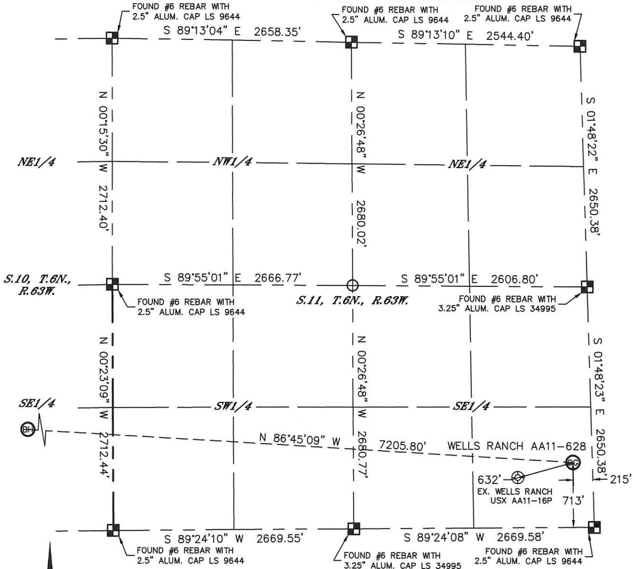
In accordance with a request from Greg Wilson with Noble Energy Inc. Lat40°, Inc. has determined the surface location of the WELLS RANCH AA11-62B to be 713' from the SOUTH line and 215' from the EAST line of Section 11, Township 6 North, Range 63 West and the bottom hole to be 1197' from the SOUTH line and 2085' from the EAST line as measured at right angles from the section lines of Section 10, Township 6 North, Range 63 West of the Sixth Principal Meridian, County of Weld, State of Colorado.
