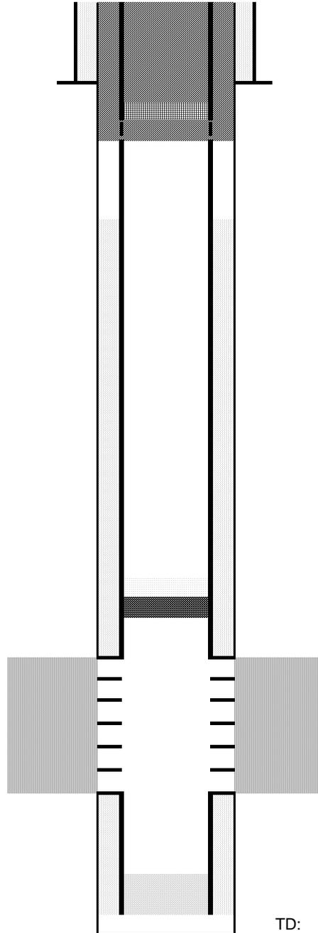
Cut surface casing off 6'-8' below surface.
