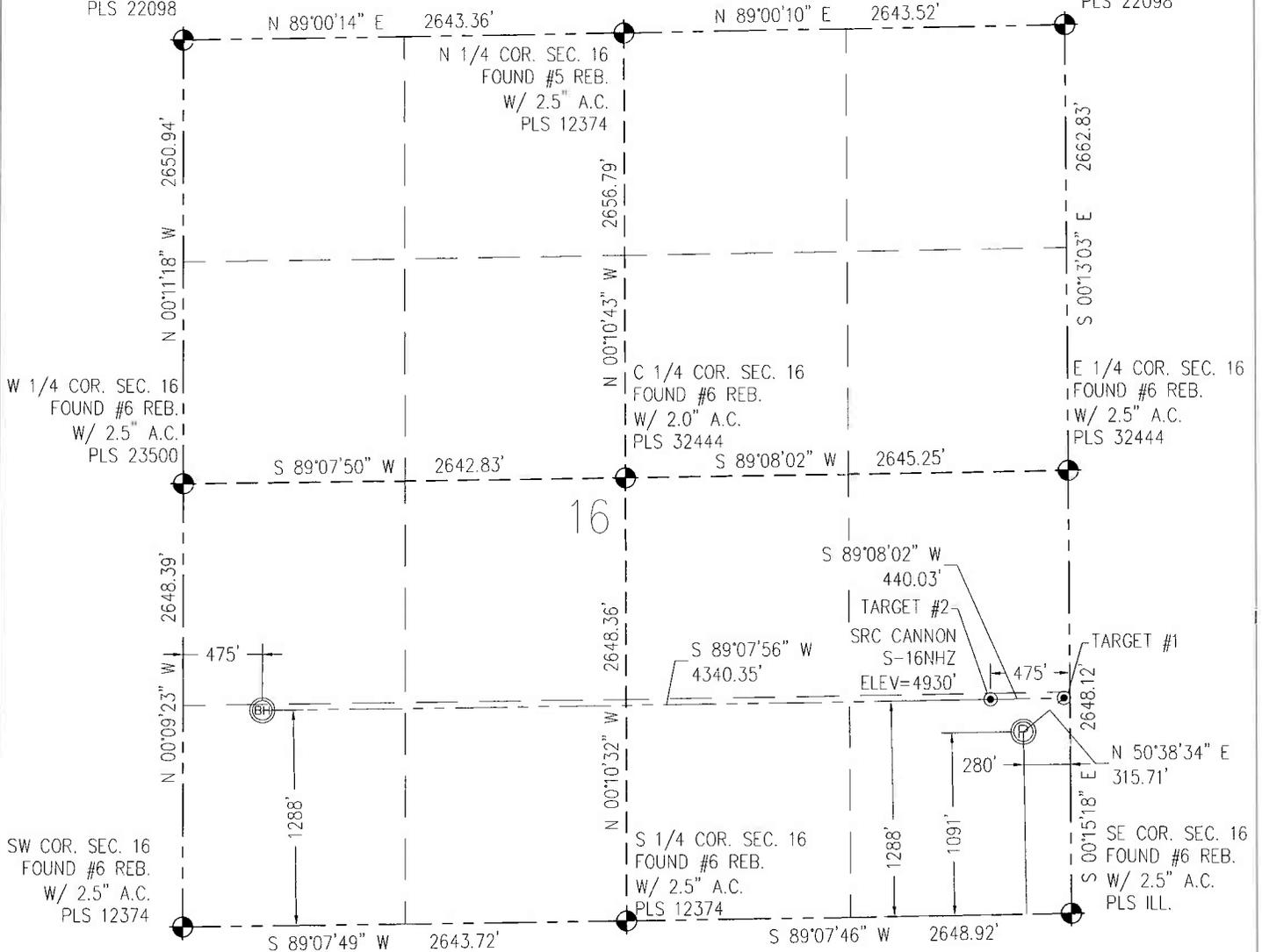
IN ACCORDANCE WITH A REQUEST FROM CRAIG RASMUSON - SYNERGY RESOURCES, BASELINE ENGINEERING CORP. HAS DETERMINED THE LOCATION OF THE SRC CANNON S-16NHZ TO BE 1091' FSL AND 280' FEL, AS MEASURED AT NINETY (90) DEGREES FROM THE SECTION LINE OF SECTION 16, TOWNSHIP 4 NORTH, RANGE 68 WEST AND THE BOTTOM HOLE LOCATION TO BE 1288' FSL AND 475' FWL OF SECTION 16, TOWNSHIP 4 NORTH, RANGE 68 WEST, 6TH PRINCIPAL MERIDIAN, WELD COUNTY, COLORADO.
